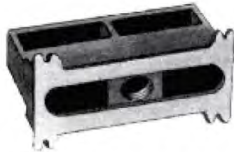
Cast Iron Adjustable Insert Used to stabilize Stone which is otherwise supported. Allows for horizontal adjustment. Can be used to hang soffit stones.
